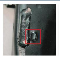
Fig. 14. Rectangular clinched joint used for the preliminary fixing of parts before their final bonding
