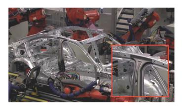
Fig. 25. The B-pillar, made of high-strength steel, of the BMW 3 car
