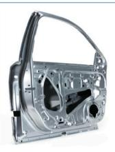
Fig. 22. Steel and aluminium door structure of a Honda motor vehicle
