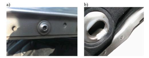
Fig. 23. Clinched joints in a Mercedes C-class: a) - fragment of the bonnet; b) - fragment of the boot lid
