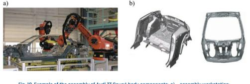
Fig. 10. Example of the assembly of Audi TT Coupé body components: a) – assembly workstation; b) – body components assembled with the use of the CL technology
