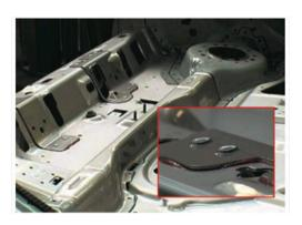
Fig. 28. Hybrid joint between sheet metal components of the Mercedes S-class body
