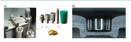
Fig. 6. Example joint-forming tools (a) and the cross-section of a joint formed with the use of a round solid die (b): 1 – punch in a blank-holding sleeve with a spring; 2 – elastomer ring of the die with movable segments; 3 – blank-holding elastomer sleeve
